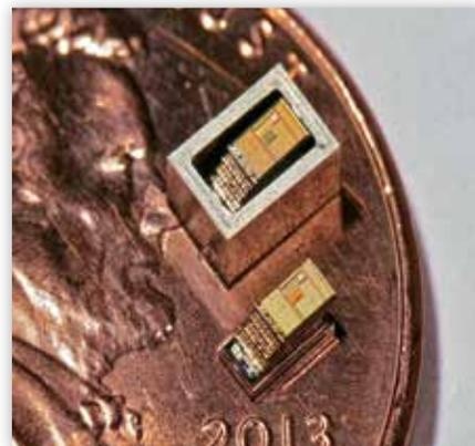
Advanced Energy Consortium's first-generation prototype multisensing microsystems shown here were developed by a team at the University of Michigan.
